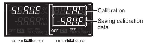
Display for saving calibration data (blinking)
